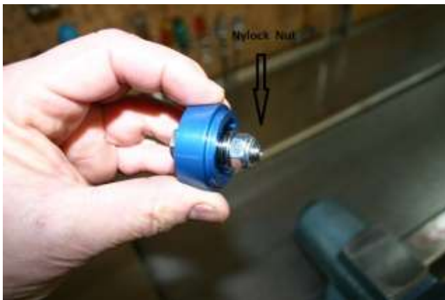
The Nylock Nut down into the fork.
